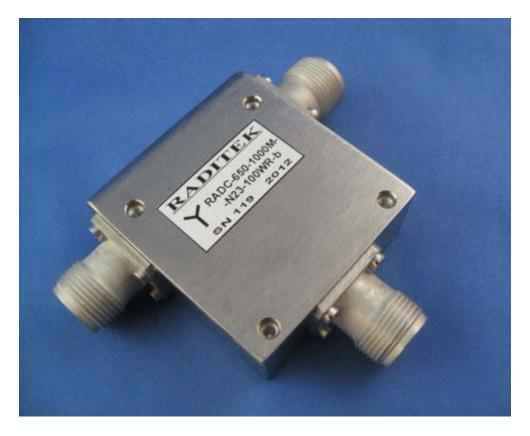
RADITEK'S Compact Wide Bandwidth Coaxial Circulator operating from 650-1000MHz at 100Watts. The RADC-650-1000M-N23-100WR-b, is a 650-1000MHz coaxial circulator with N-Type female connectors and 100 watts of power handling. Specifications: 0.8 dB Insertion Loss, 14dB Isolation, 1.60:1 VSWR Dimensions: 48.5(W) x 53.5(L) 20.8(T) mm.. The unit connects direct to any WAN/LAN, with TCP and HTTP acceleration, data compression
